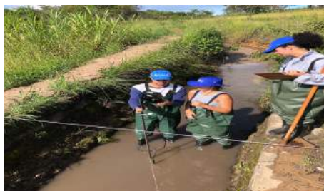
(c) Measurement with the Flowtracker
