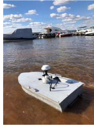
(b) Boat design and built to remote operate the M9
